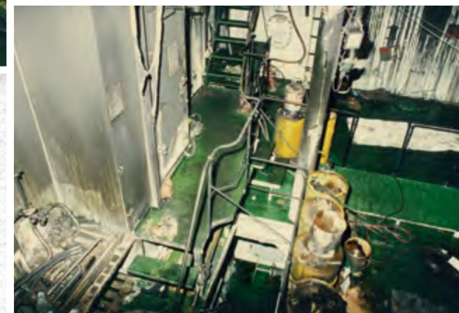
TOP: After the fire aboard the British Adventure, much of the items in the steering gear room (where the fire occurred) was covered in soot.
