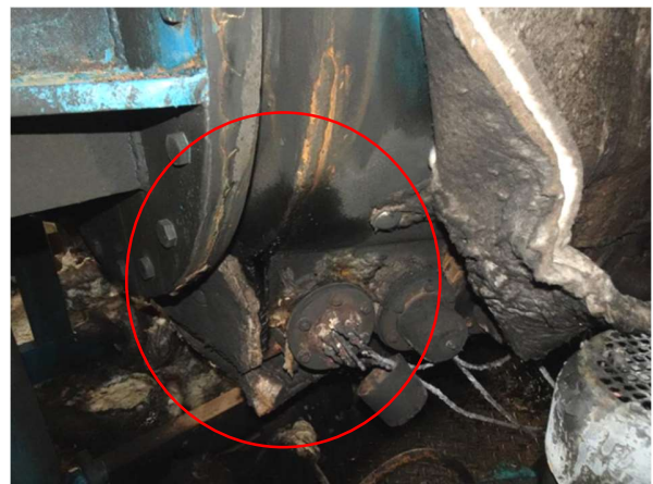
Figure 38: Dark stain on oil jacket, circled in red
