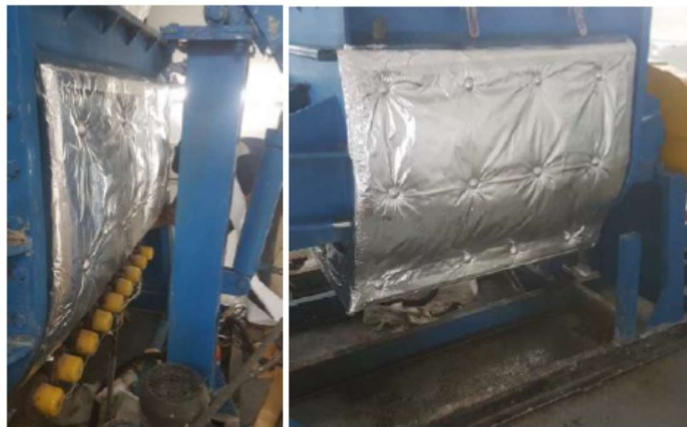
Figure 18: Photographs of the insulation on the oil jacket taken by Marimuthu on 6 February 2021
