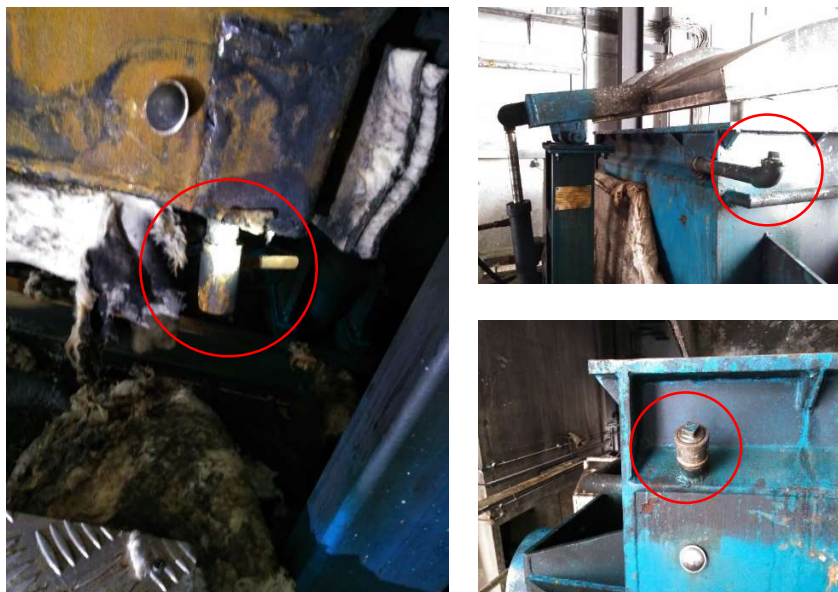
Figure 40: All three openings on the oil jacket circled in red were found closed
