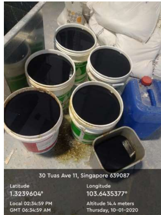
Figure 15: A total of six containers of darkened used oil were drained from the oil jacket
