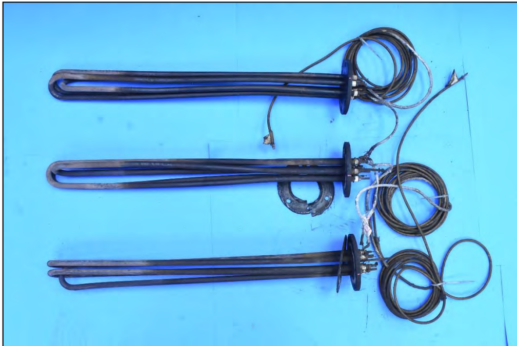
Figure 90: All the gaskets had degraded and were generally brittle to the point where they broke with slight pressure. Some broke during the removal of heaters.
