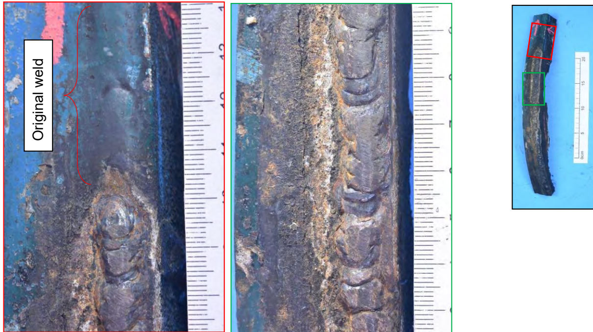
Figure 51: Close up view of side weld. Part of the original weld is indicated (in red) in the left figure. The rest of the weld was repaired and had a face width of about 20 mm.
