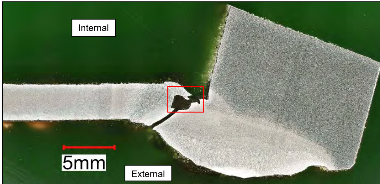
Figure 169: Sectional metallographic examination was conducted across the repair weld which had cracked through. Voids up to about 1.5 mm wide were in the weld metal (red box).
