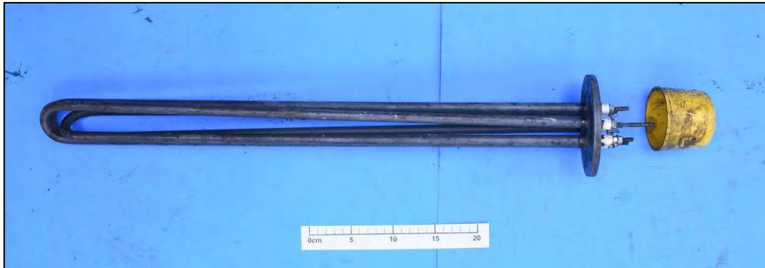
Figure 111: Heater found on the Platform beside the Mixer Machine. No significant damage was observed.
