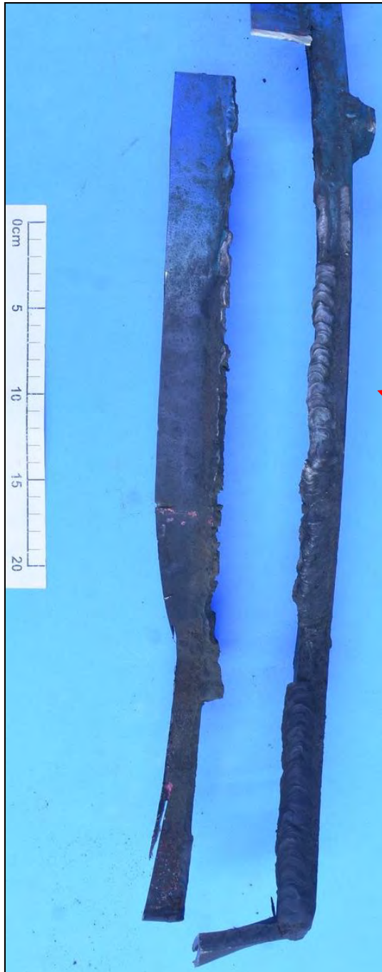
Figure 65: Cut out section of the rear side, right edge weld. The observations made in the following figures were generally similar to the rear side, left edge weld. (see also Figure 62)
