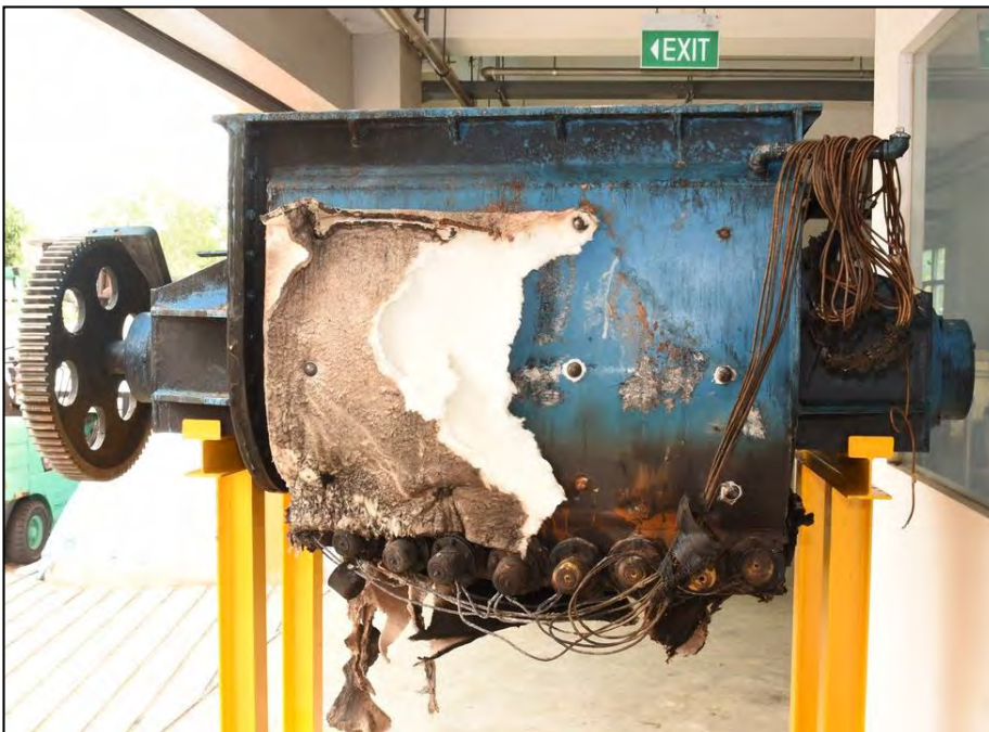
Figure 22: As-received condition of the Mixer Machine from the rear.
