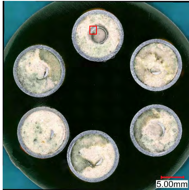
Figure 201: Sectional metallographic examination was conducted across metal tubes of new heater.
