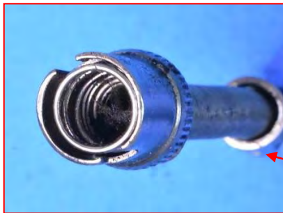
Figure 102: RTD B remnants retrieved onsite. Although this RTD was not attached to the electrical panel during the onsite inspection, the wires were originally connected to the “Material temp” thermostat as the connectors were still in place inside the panel. See Figure 107.
