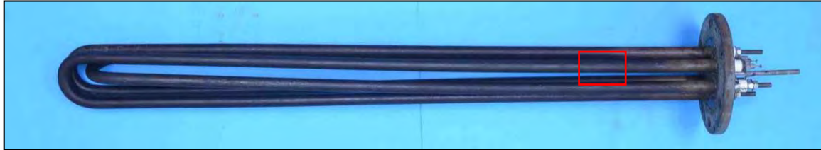
Figure 205: The used heater with blisters were sectioned across one of the blister.
