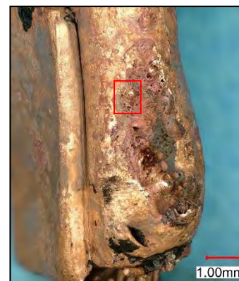
Figure 135: SEM confirms the arcing characteristic with large percentage of voids.
