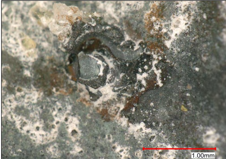
Figure 95: At the metal tube inner diameter wall corresponding to the location of the separated wire, a small melted bulb was observed adhering to the wall. .
