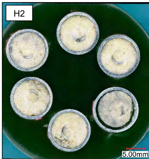
Figure 181: Heaters #2, #5 and #8 were sectioned 10 cm from the end of the heaters, across the metal tubes as shown in example above for metallographic examination. A new heater was sectioned the same way for comparison.
