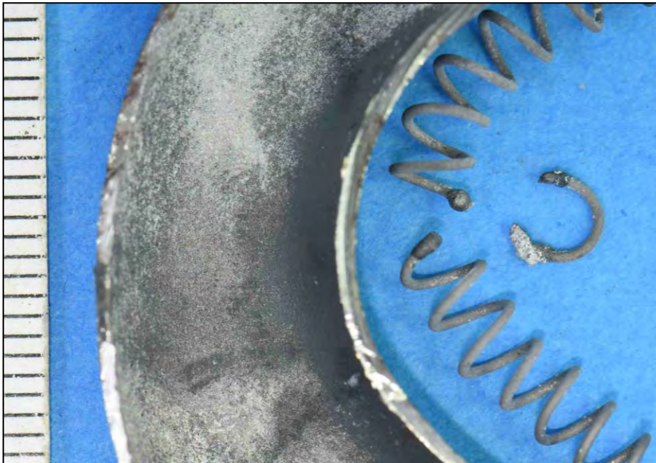
Figure 96: The tips of the wire had melted with some of the insulation powder fused onto the tip.
