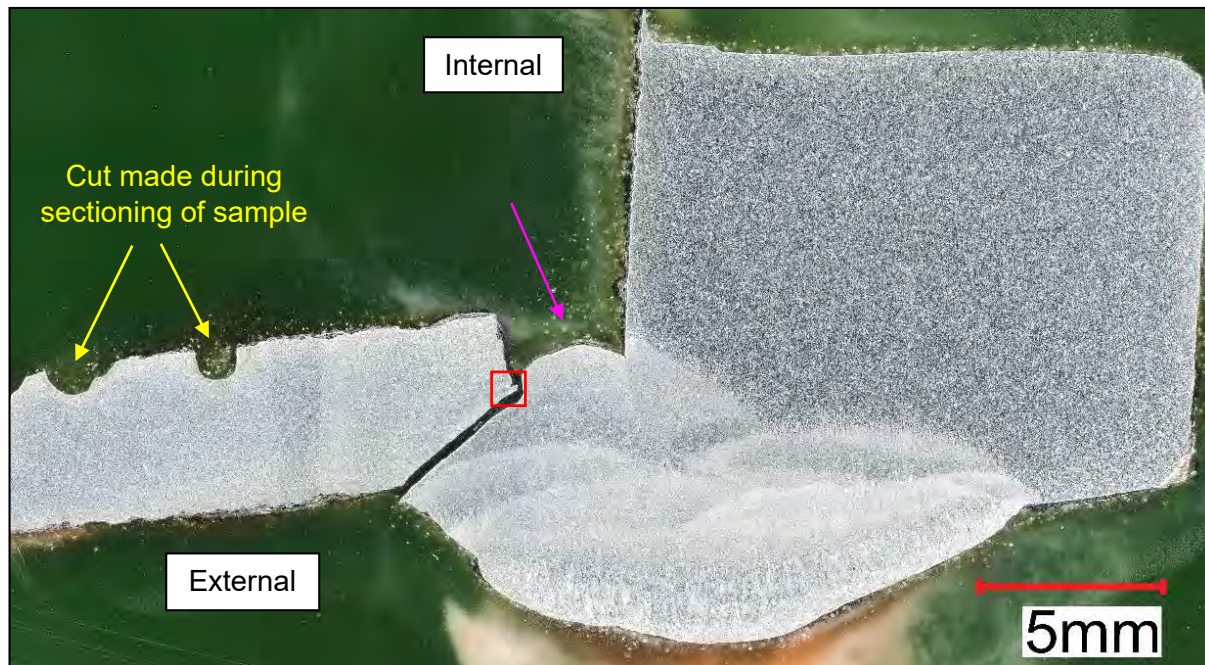
Figure 171: Sectional metallographic examination was conducted across the repair weld and through crack. The weld had lack of root penetration with root opening of about 3.0 mm wide (pink arrow).
