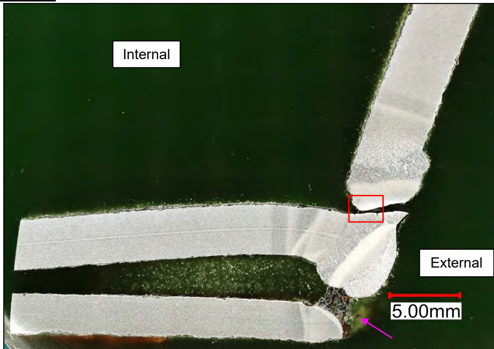
Figure 175: Sectional metallographic examination was conducted across the weld between the bottom plate and reinforcement plate. A through-thickness void was observed at the weld joint of the reinforcement plate (pink arrow).
