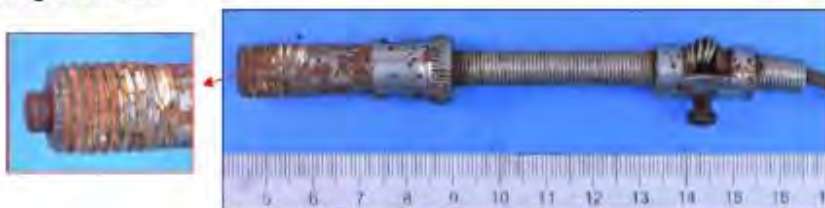
RTD A with working sensor on left.
