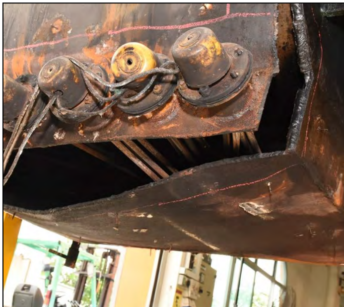
Figure 58: Marked out locations on the rear edges and corners for detailed examination.
