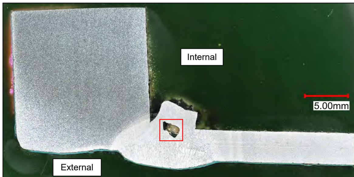
Figure 147: Section metallographic examination was conducted across the original weld. Excessive root penetration was observed at this weld area. About 2 mm width void was observed in the middle of the weld root.
