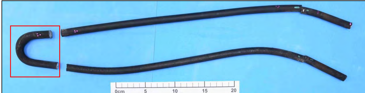
Figure 93: The LEW reported that heater #2 had unusual high resistance among the coils. With that reporting, the metal tubes were examined and the tube between terminals #3 and #6 were found to have a bulged area.
