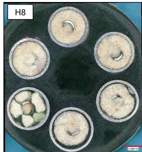
Figure 181: Heaters #2, #5 and #8 were sectioned 10 cm from the end of the heaters, across the metal tubes as shown in example above for metallographic examination. A new heater was sectioned the same way for comparison.
