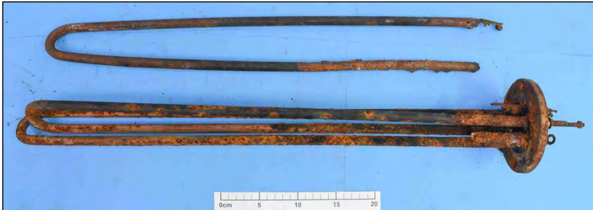
Figure 113: Used heater that were replaced after failure (received for analysis on 28th May 2021). This heater was reportedly replaced in August 2020 after it failed.
