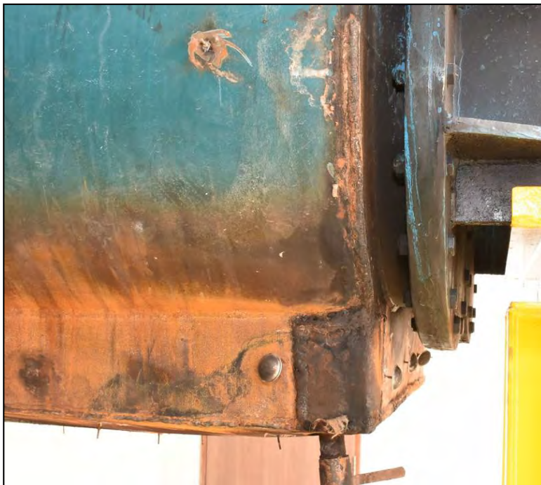
Figure 26: As-received condition of the Mixer Machine as seen from the front right bottom corner.
