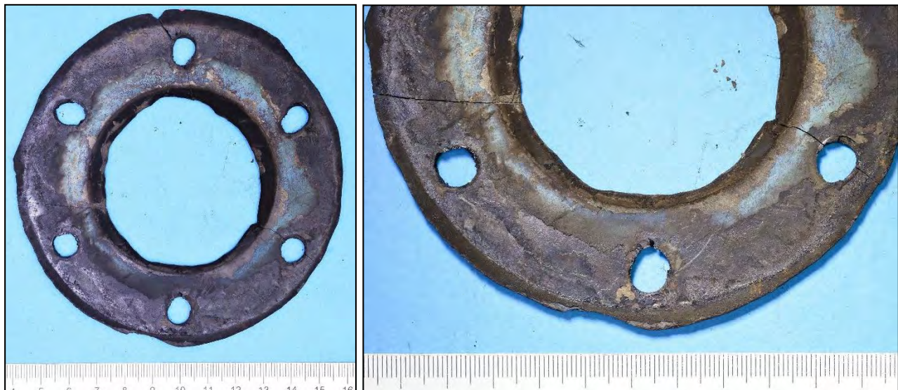
Figure 92: For comparison, gasket for heater #9 which was located furthest from the main rupture zone and heater #2, was selected to undergo shore hardness testing. Similarly, parts of it were broken during the testing.
