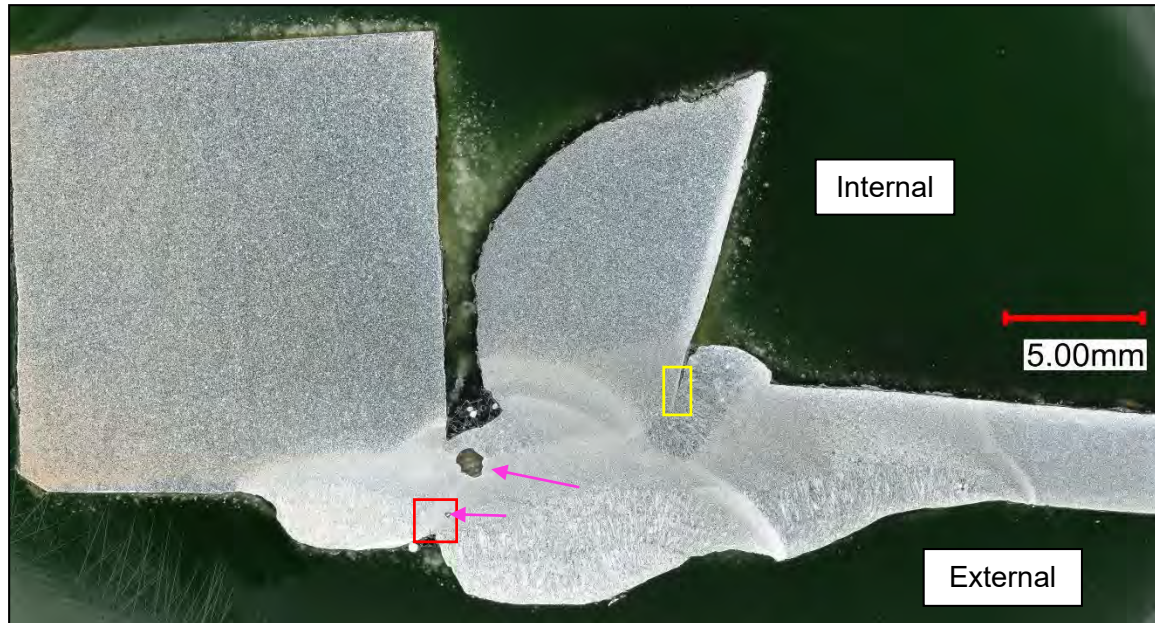
Figure 151: Sectional metallographic examination was conducted across the repair weld with a visible insert plate from the internal side (see Figure 47). Voids up to about 1.0 mm were observed (in pink).
