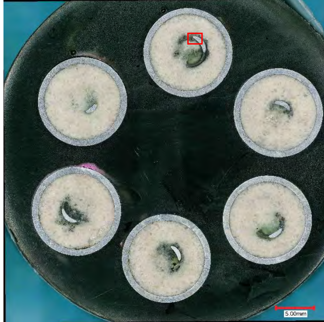
Figure 189: Sectional metallographic examination was conducted across metal tubes of heater #5.
