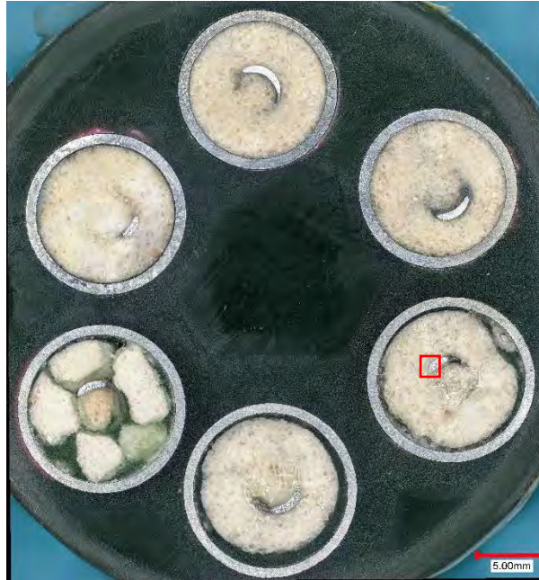
Figure 195: Sectional metallographic examination was conducted across metal tubes of heater #8.
