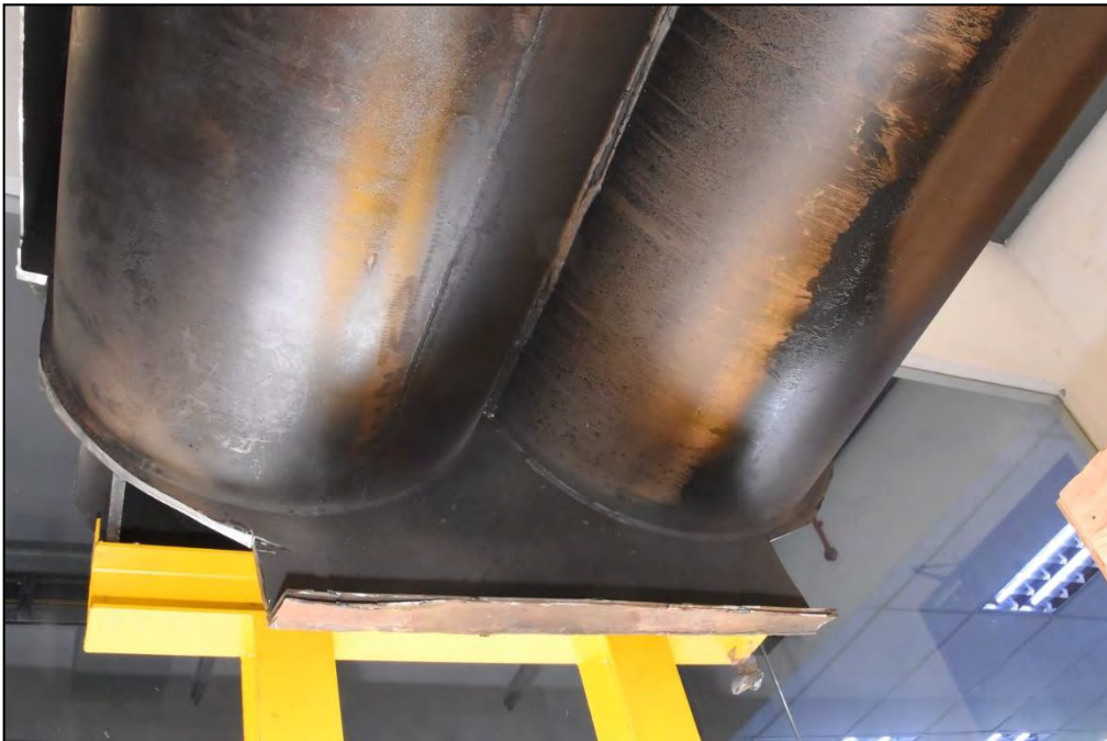
Figure 74: Internal condition of the oil jacket surface, view from the bottom. Surface was generally covered with soot and oil remnant.
