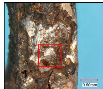
Figure 139: SEM confirms the arcing characteristic with concentric rings observed to be emanating from the centre of the arcing damage.
