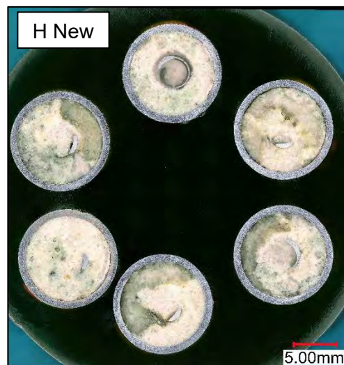
Figure 182: Cross sections for heater #2 (abbreviated as H2), heater #5 (abbreviated as H5), heater #8 (abbreviated as H8), new heater (abbreviated as H New).
