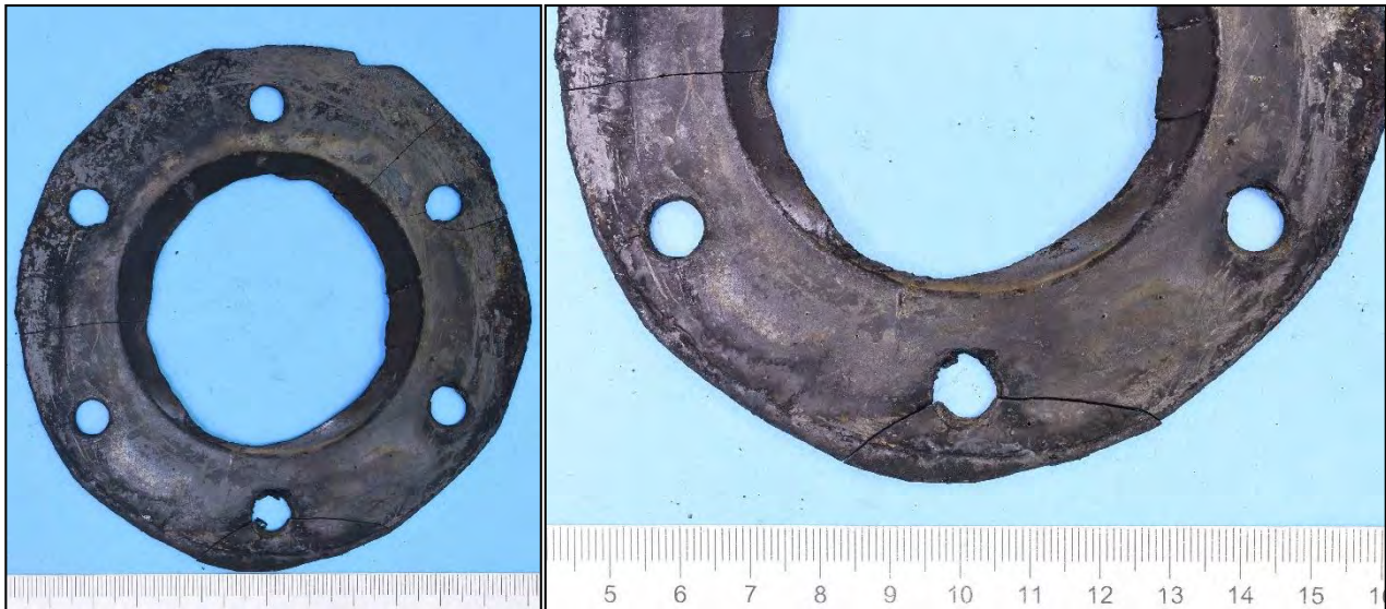
Figure 91: General view of gasket for heater #2. Some parts were broken during the shore hardness testing.
