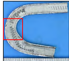
Figure 95: At the metal tube inner diameter wall corresponding to the location of the separated wire, a small melted bulb was observed adhering to the wall. .
