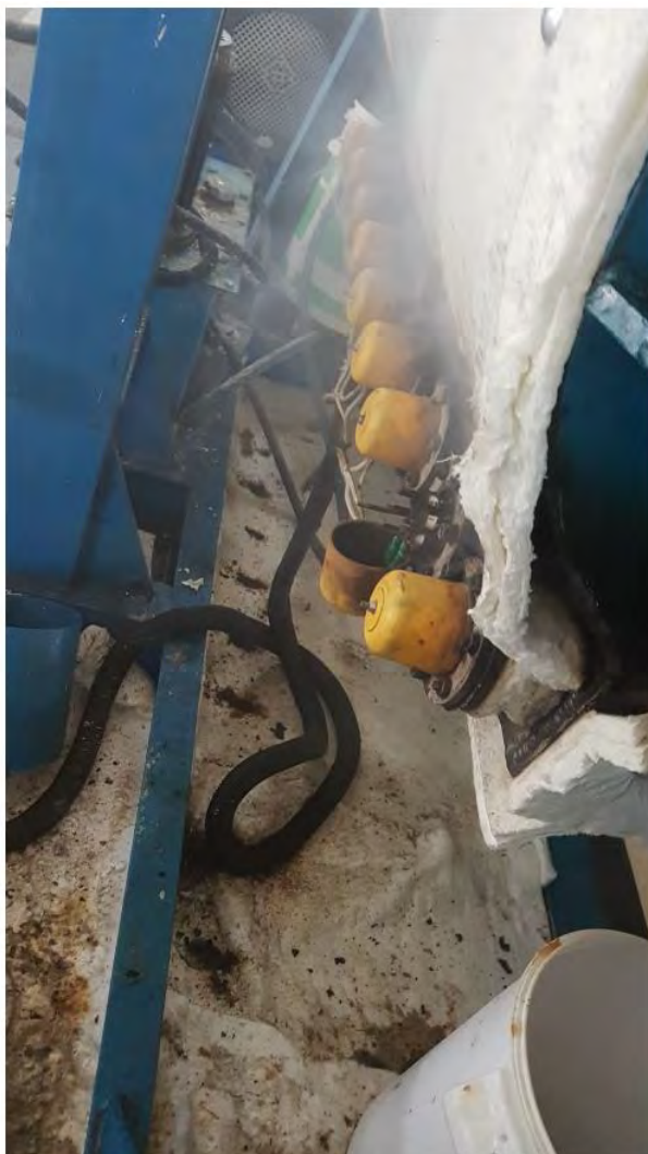
S-83: Photograph taken by Marimuthu on 24 February 2021 at 11:13am showing that the wiring of the damaged Heater No. 2 had been taped together with green tape, extracted from Marimuthu's mobile phone
